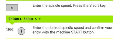
The spindle speed S with the entered rpm is started with a miscellaneous function M. Proceed in the same way to enter a miscellaneous function M.
