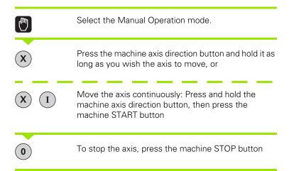
You can move several axes at a time with these two methods. You can change the feed rate at which the axes are traversed with the F soft key, see "Spindle speed S, feed rate F and miscellaneous functions M", page 567.
