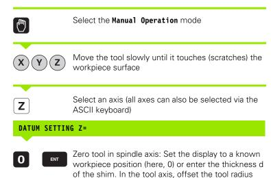
Repeat the process for the remaining axes.
