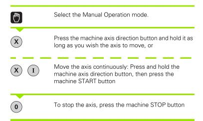
You can move several axes at a time with these two methods. You can change the feed rate at which the axes are traversed with the F soft key, see "Spindle speed S, feed rate F and miscellaneous functions M", page 479.
