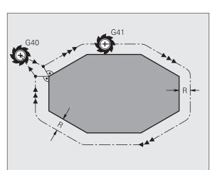
For radius compensation, the TNC takes the delta values from both the  ${\bf T}$  block and the tool table into account:
