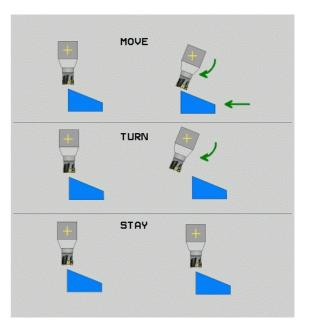
▶ Dist. tool tip – center of rot. (incremental): The TNC tilts the tool (or table) relative to the tool tip. The SET UP parameter shifts the center of rotation of the tilting movement relative to the current position of the tool tip.
