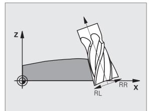
12.5 Peripheral milling: 3-D radius c<mark>om</mark>pensation with workpiece orientation
