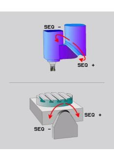
Example for a machine with a rotary table C and a tilting table A. Programmed function: **PLANE SPATIAL SPA+0 SPB+45 SPC+0**
