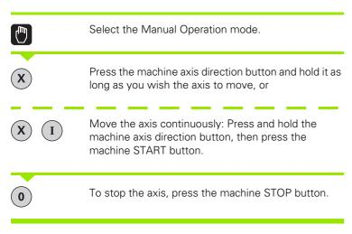
You can move several axes at a time with these two methods. You can change the feed rate at which the axes are traversed with the F soft key, see "Spindle Speed S, Feed Rate F and Miscellaneous Functions M", page 462.
