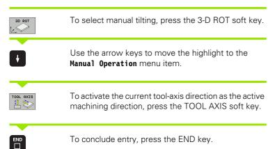
To reset the tilting function, set the **Manual Operation** menu item in the "Tilt working plane" menu to inactive.
