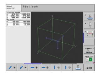
You can also activate the working-space monitor for the Test Run mode in order to test the program with the current datum and the active traverse ranges (see table below, last line).
