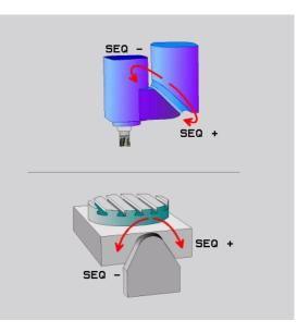
Example for a machine with a rotary table C and a tilting table A. Programmed function: **PLANE SPATIAL SPA+0 SPB+45 SPC+0**
