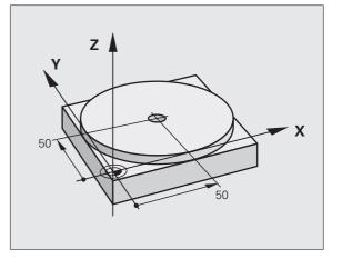
First you pre-position the tool with straight-line blocks to the hole center coordinates at a setup clearance of 5 mm above the workpiece surface. Then drill the hole with Cycle **G200**.
