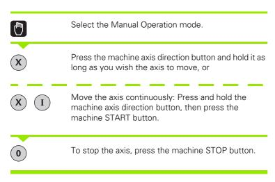
You can move several axes at a time with these two methods. You can change the feed rate at which the axes are traversed with the F soft key, see "Spindle Speed S, Feed Rate F and Miscellaneous Functions M," page 440.
