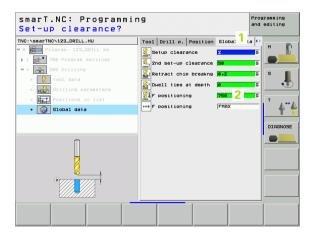
Changing a global parameter on the **global data** detail form only effects a local change of the parameter, valid for that one machining step. smarT.NC displays the input fields of locally changed parameters with a red background. On the right side of the input field is an **L** which identifies the value as valid **locally**.
