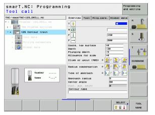
Contour name: Name of the contour file (.HC) to be machined. If the DXF converter option is available, you can use it to make a contour directly from the form.
