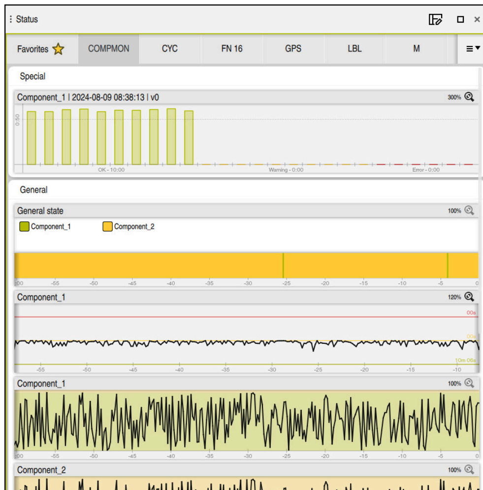
The COMPMON tab with configured spindle speed monitoring
