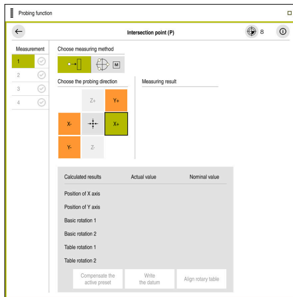
Probing function workspace with an open manual probing function
