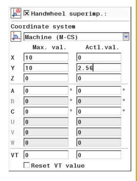
By entering values in the **Max. val.** column, you define which axes may be moved using the handwheel and the maximum path by which they may be moved. Since the input value applies to both directions (both positive and negative), the maximum path is double the input value.
