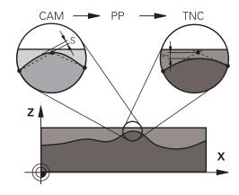
Adapt the chord error in the CAM program, depending on the machining:
