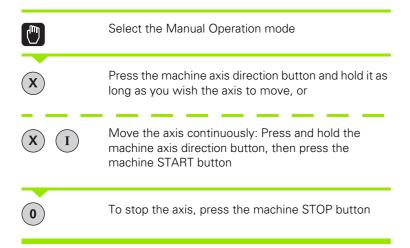
You can move several axes at a time with these two methods. You can change the feed rate at which the axes are traversed with the F soft key, see "Spindle Speed S, Feed Rate F and Miscellaneous Functions M", page 370.
