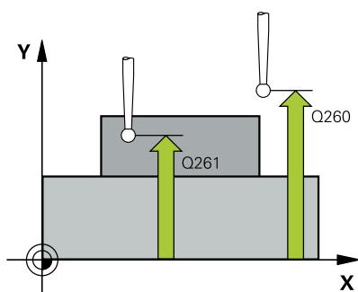
**說明圖****Parameter****Q260 Clearance height?**
