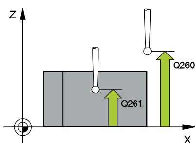
**說明圖****Parameter****Q260 Clearance height?**
