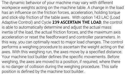
In addition to adjusting the control parameters, with LAC the maximum acceleration is also adjusted in accordance with the weight. This enables the dynamics to be accordingly increased with low load to increase productivity.
