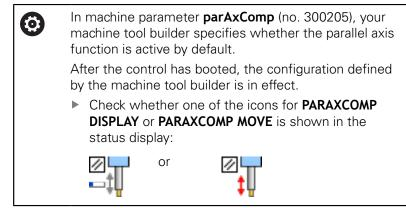
If the machine tool builder has already enabled the parallel axis in the configuration, the control takes this axis into account in the calculations, without you having to program **PARAXCOMP**.
