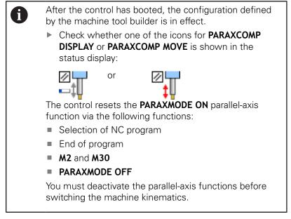
Use the **PARAXCOMP OFF** function to switch off the parallel-axis function. The control then uses the principal axes defined by the machine tool builder.
