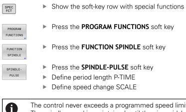
The control never exceeds a programmed speed limit. The spindle speed is maintained until the sinusoidal curve of the **S-PULSE FUNCTION** falls below the maximum speed once more.
