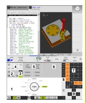
Operating panel of the Test Run mode
