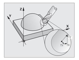
Example: Block format with surface-normal vectors without tool orientation
