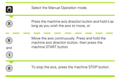
You can move several axes at a time with these two methods. You can change the feed rate at which the axes are traversed with the F soft key (see "Spindle Speed S, Feed Rate F and Miscellaneous Functions M," page 52).
