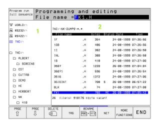
It may take some time to mount a network device. At the upper right of the screen the TNC displays [**READ DIR**] to indicate that a connection is being established. The maximum data transmission rate lies between 200 and 1000 kilobaud, depending on the file type being transmitted.
