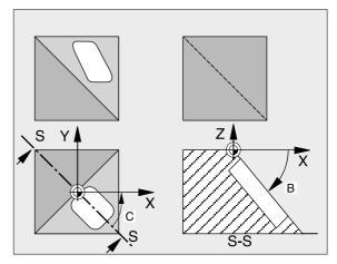
If you set the function TILTING program run to ACTIVE in the Manual Operation mode see "Tilting the working plane," page 24, the angular value entered in this menu is overwritten by Cycle 19 WORKING PLANE.
