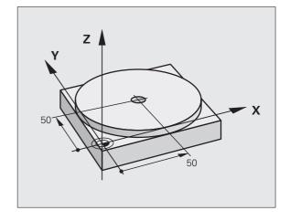
First you pre-position the tool with straight-line blocks to the hole center coordinates at a setup clearance of 5 mm above the workpiece surface. Then drill the hole with Cycle **G200**.
