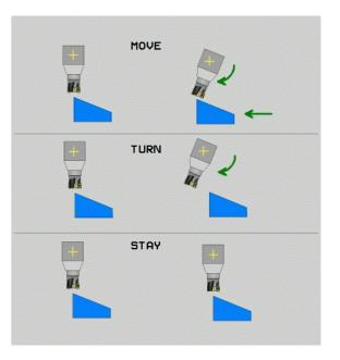
▶ Dist. tool tip – center of rot. (incremental): The TNC tilts the tool (or table) relative to the tool tip. The DIST parameter shifts the center of rotation of the positioning movement relative to the current position of the tool tip.
