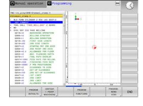
After pressing the **SPEC FCT** key, you can open the **smartSelect** selection window with the **GOTO** key. The control displays a structure overview with all available functions. You can rapidly navigate with the cursor or mouse and select functions in the tree diagram. The control displays online help for the selected function in the window on the right.
