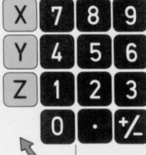
Selection of appropriate axis by pressing the axis keys
