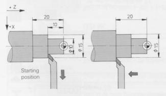
X axis is in diameter display mode.
