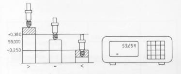
The measured value display can output the tolerance status through two lines for external subsequent processing (see "remote operation" in the operating instructions).
