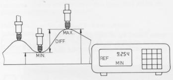
The maximum/minimum acquisition occurs every 0.55 ms. Maxima and minima occurring between these acquisitions are not detected. Therefore the test specimen must be moved in such a way that the change in measured values within 0.55 ms is less than the desired accuracy.
