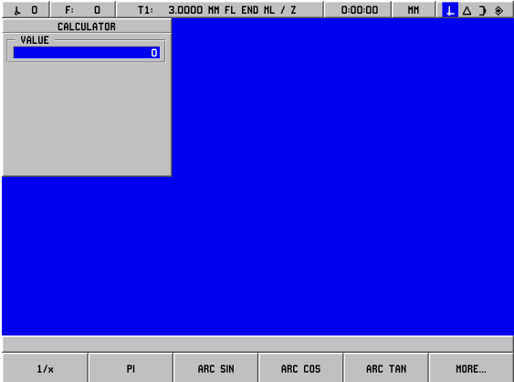
Fig. I.70 Trig function soft keys
