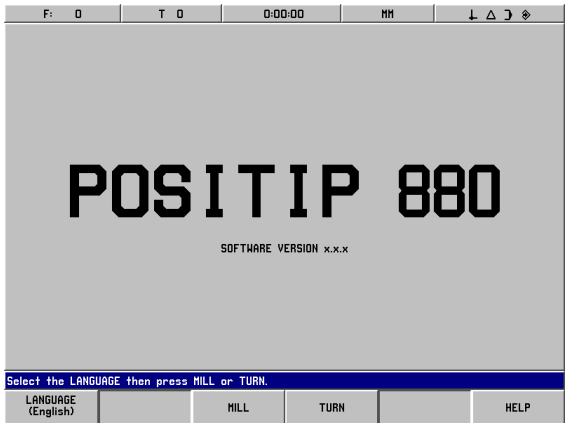
Fig. II.6 POSITIP 880 screen after initial switch-on
