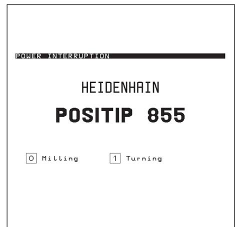
Fig. 37: POSITIP screen after initial switch-on
