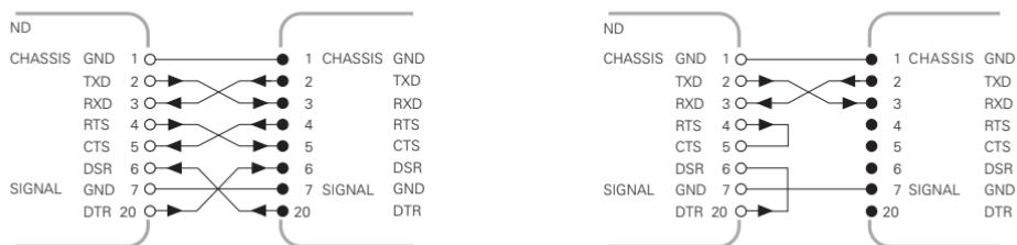
**CHASSIS GND:** Chassis Ground; **TXD:** Transmitted Data, **RXD:** Received Data, **RTS:** Request To Send, **CTS:** Clear To Send; **DSR:** Data Set Ready; **SIGNAL GND:** Signal Ground; **DTR:** Data Terminal Ready
