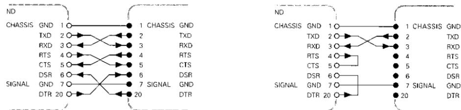
**CHASSIS GND:** Chassis Ground; **TXD:** Transmitted Data, **RXD:** Received Data, **RTS:** Request To Send, **CTS:** Clear To Send; **DSR:** Data Set Ready; **SIGNAL GND:** Signal Ground; **DTR:** Data Terminal Ready
