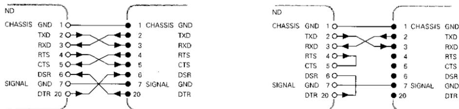
**CHASSIS GND:** Chassis Ground; **TXD:** Transmitted Data; **RXD:** Received Data;
