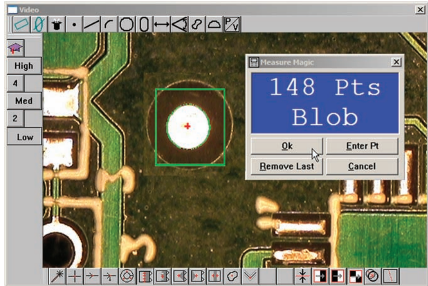
The Blob probe is used to measure a solder pad
