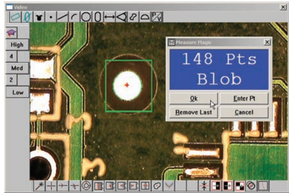
One hundred and forty eight points are acquired by the Blob probe to measure a solder pad
