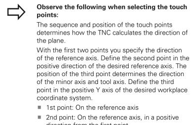
3rd point: On the minor axis, in a positive direction of the desired workpiece coordinate system
