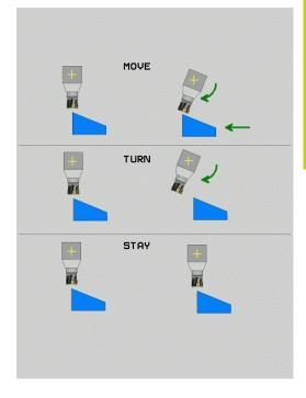
You will position the rotary axes later in a separate positioning block
