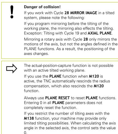
The TNC only supports tilting the working plane with spindle axis Z.
