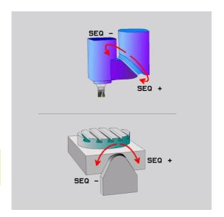
Example for a machine with a rotary table C and a tilting table A. Programmed function: **PLANE SPATIAL SPA+0 SPB+45 SPC+0**
