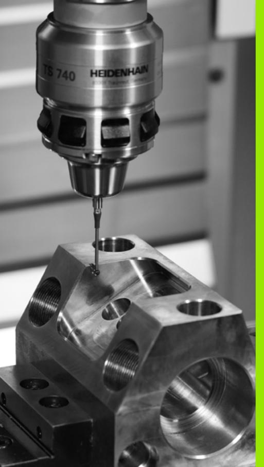
Touch Probe Cycles: Automatic Measurement of Workpiece Misalignment
